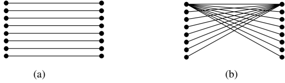
Fig. 3. Two examples of bipartite graphs with n = 2^W = 8 (for W = 3 ) vertices in each graph side representing two two-column FIB tables A_1 and A_2 . In the first graph (a), there is a perfect match and the size of the (minimal) edge cover is 8 = n = \alpha \cdot n with \alpha = 1 and OPT(A_1) = 2W = 6 . In the second (b), the size of the edge cover is 14 = \alpha \cdot n with \alpha = 1.75 and OPT(A_2) \geq 5 .
