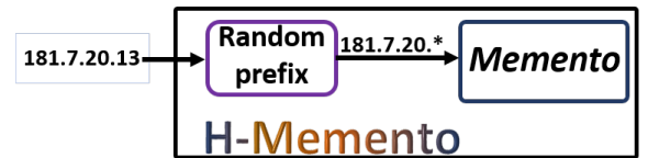
(b) Our HHH algorithm, H-Memento , simply updates Memento with a single random prefix, achieving constant time complexity.
